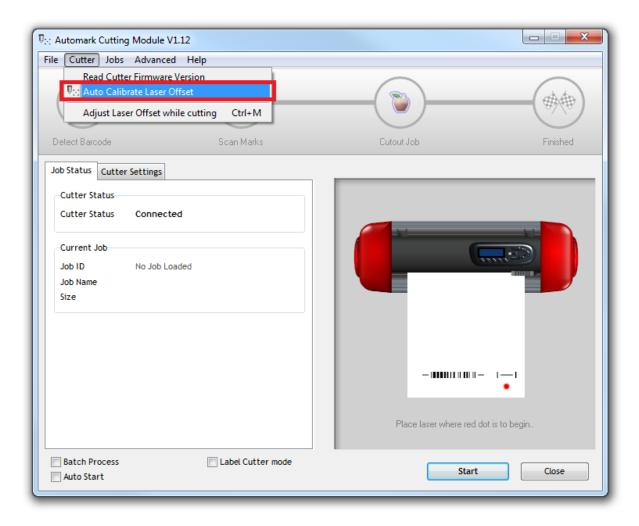
Do the Laser Calibration to measure the laser offset, and store the result in the cutter memory.
