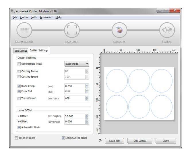
In this screen, you can select the settings you wish to use. For items such as force and speed, if you leave these settings unchecked, the current settings on the machine will be used.
