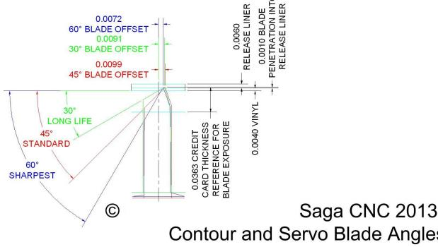
Contour and Servo Blade Angles (Based on actual blade measurements)
